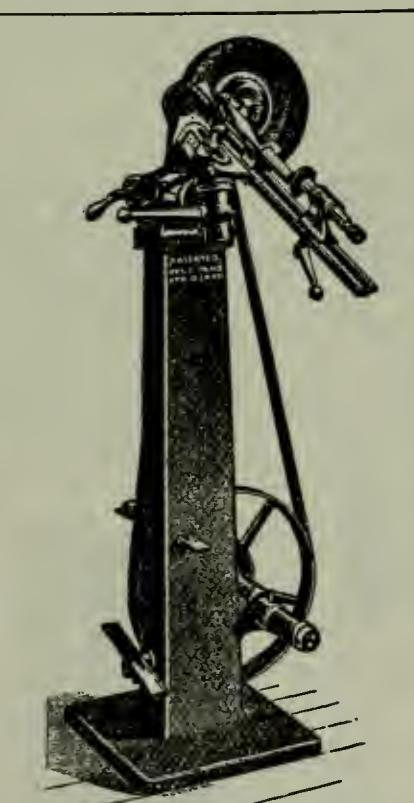
A Hand-controlled, Foot-operated Twist Drill Grinding Machine. The Drill Is Revolubly Held in a Jig At the Correct Angle Against the Emery Wheel.
